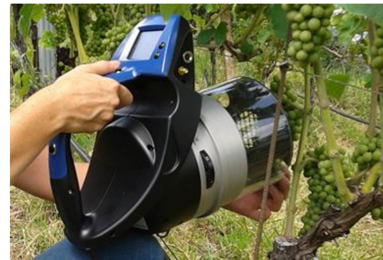
Figure 2: Fluorescence-based sensor, Multiplex® 3.6, Force-A, Orsay, France.
